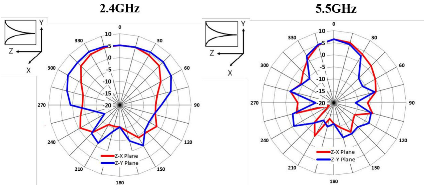
Graph5.KH-6G-0H-08 Vertical radiation pattern
