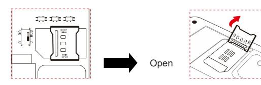
**B**Place the SIM card correctly and lock the card to the left.
